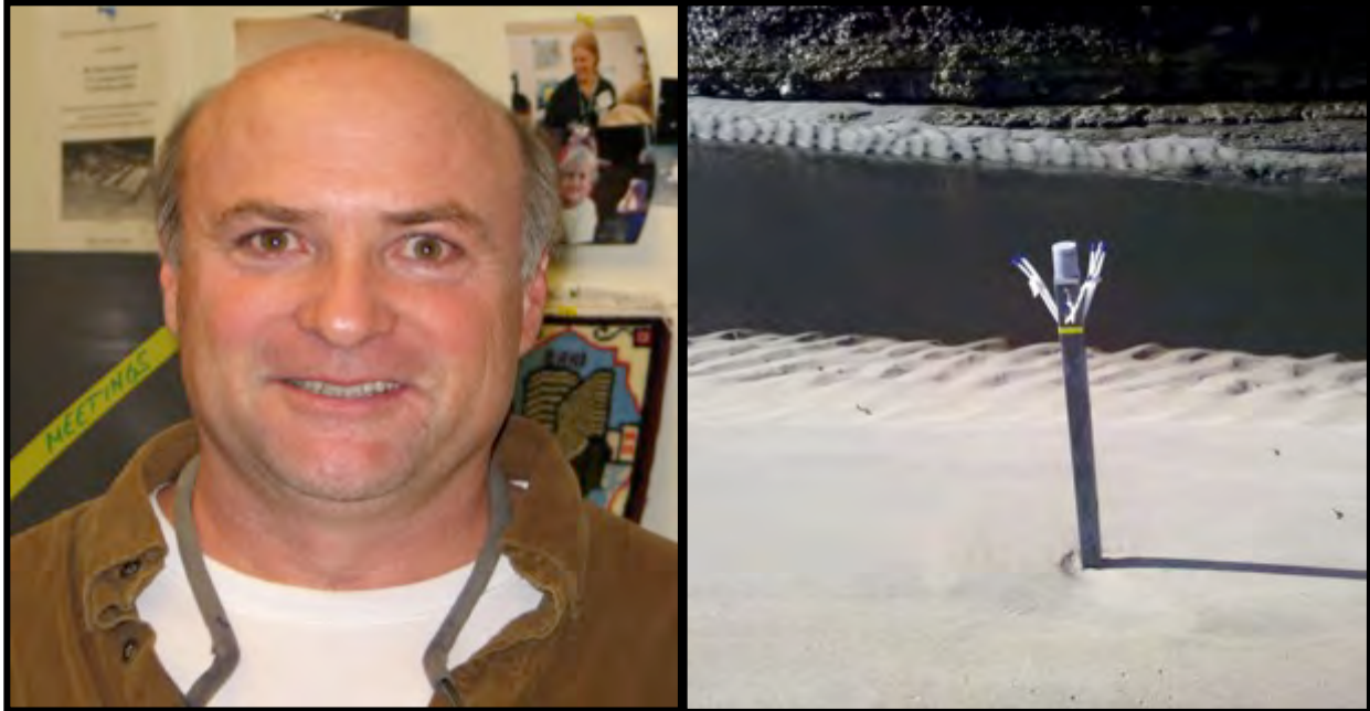
Figure 7. Dr Peter W. Swarzenski (left) and his series of temporary shallow piezometers across the YLR berm / beach face (right) (Photo courtesy USGS).
