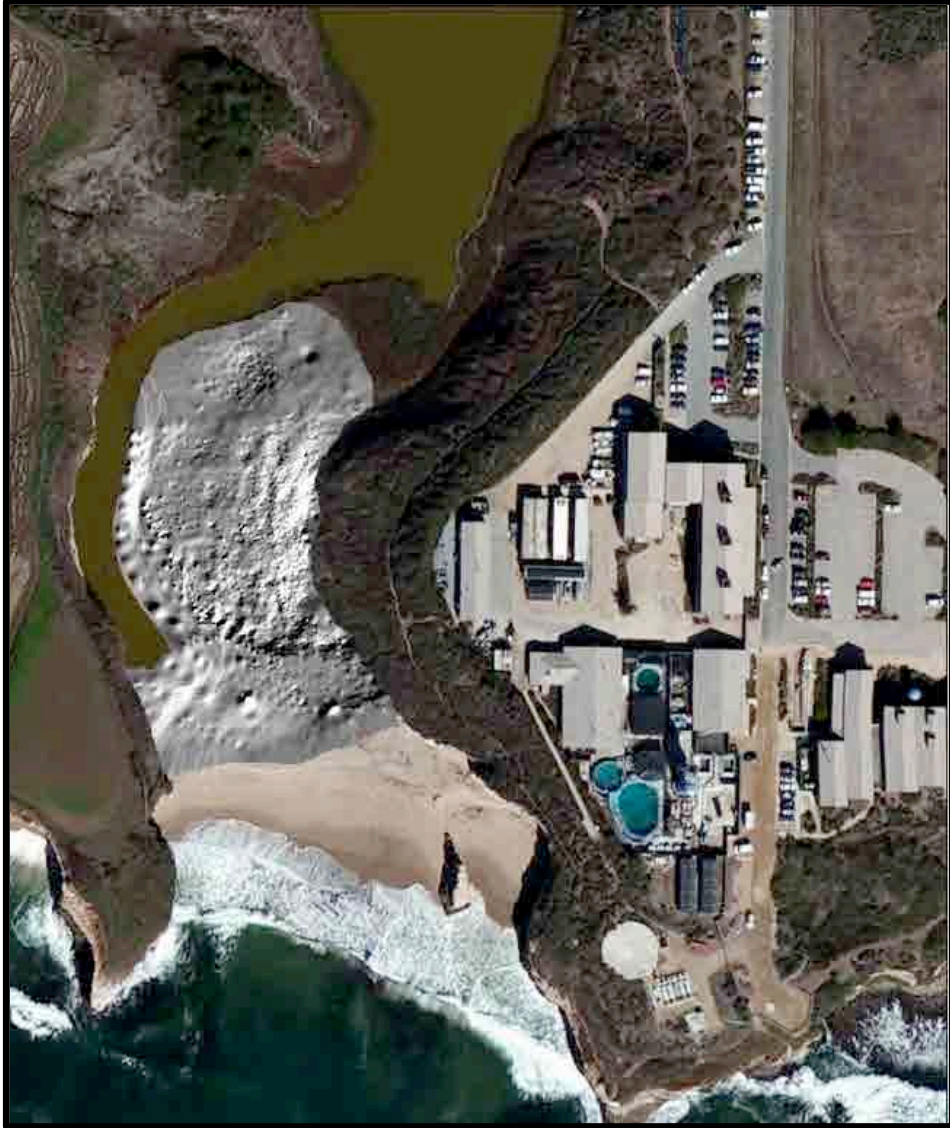
Figure 11. Younger Lagoon dune map. Survey data and resulting elevation model output shows topographic features on Younger Lagoon Beach.
