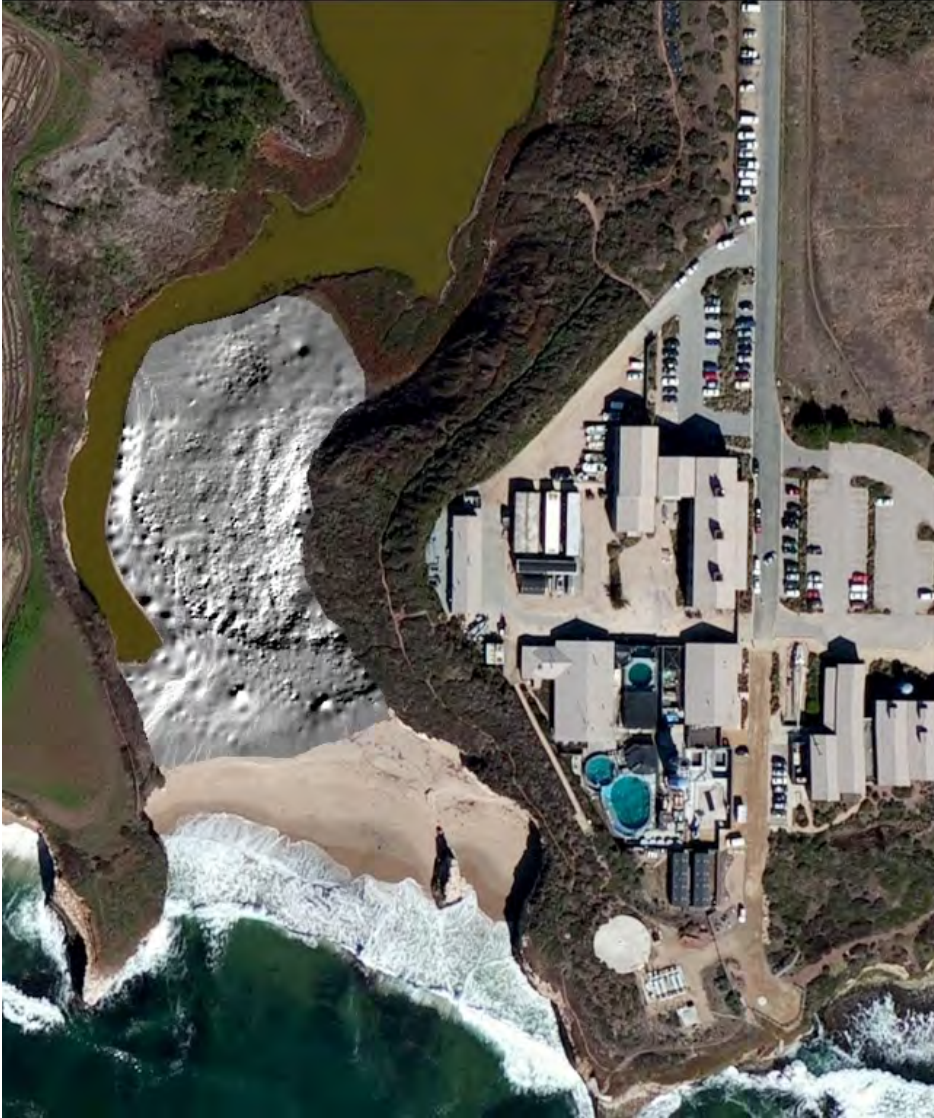
Figure 9. Younger Lagoon dune map. Survey data and resulting elevation model output shows topographic features on Younger Lagoon Beach.
